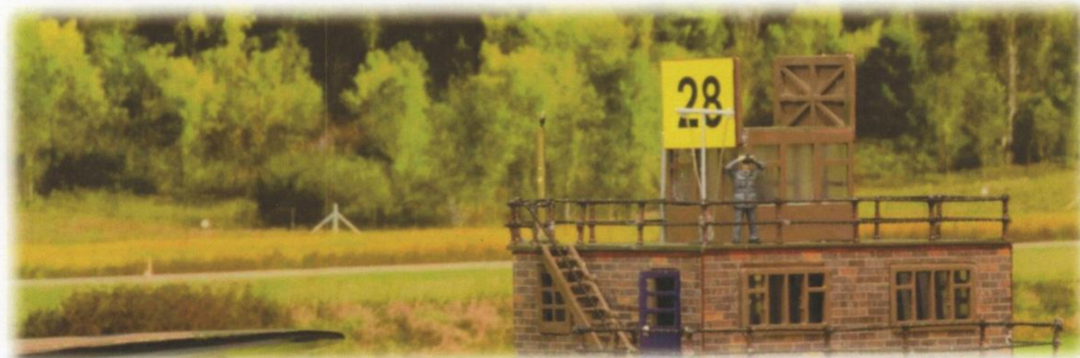
The number 28 on the landing board of the control tower guides the returning aircraft to one of three runways at RAF Linton-on-Ouse. In this case, runway 10/28, (compass heading +/- due west, 280 degrees)
