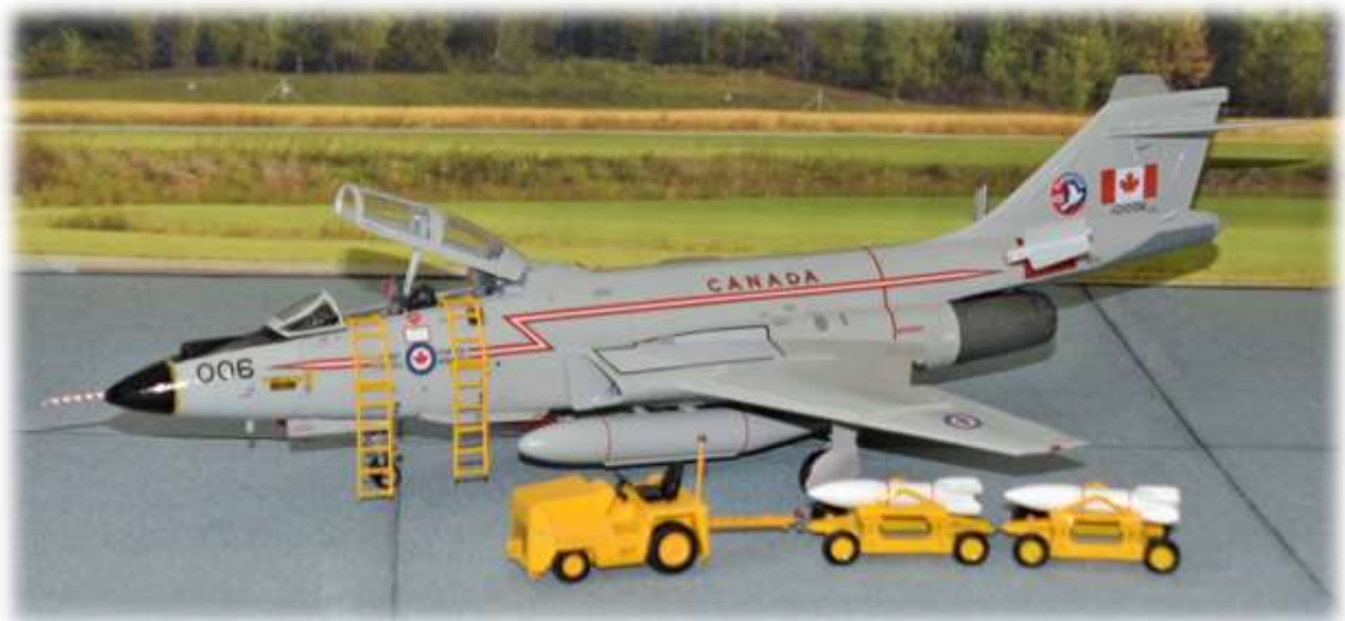
With two Genie missiles on trolleys, and tow tractor
